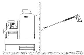
Make a partition between the wash area and the pressure washer to prevent direct nozzle spray from coming in contact with the pressure washer. Moisture reaching the equipment will reduce the pressure washer's service life.
